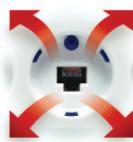
The device plugs are designed in such a way, that in the event of the the cable being pulled improperly, then the connector plug is ejected from the socket, regardless of its position (see sketch below) This prevents the cable, the connector plug itself and the socket from being broken. A so-called “disconnection call” is generated in the system. It is possible to reconnect the connector plug at any time.
